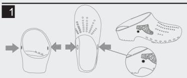
Use a 2mm punching tool to punch a hole in the side of the clog just below the right end of the "Calzuro" logo and above the front of the heel. Repeat this procedure on the other side of the clog, making certain that this hole is symmetrical with the other one.
