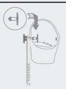
Attach the buckle on the clog on the side with the Calzuro logo by pushing it onto the post until the retention "click" is heard. Point the longend of the buckle toward the front of the clog.
